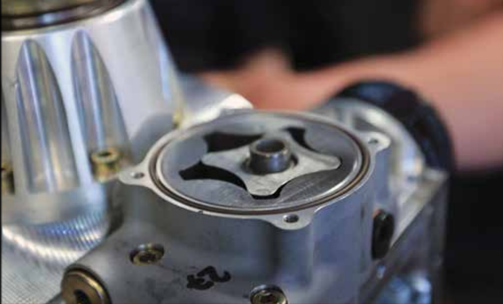
The gerotor-type oil pump is externally mounted on the front of the engine to permit easy servicing and inspection.
