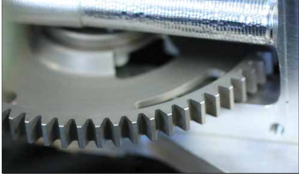
Slots machined in the starter ring gear send crankshaft position data to the ECU for ignition timing.
